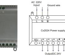
Cx2024 power supply wiring diagram
